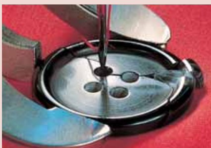
THE BUTTON CAN BE DAMAGED.
