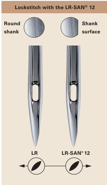
The development of the Groz-Beckert LR SAN® 12 cutting point needle has allowed an improved and more even appearance of the seams produced on twin lockstitch machines. This has been achieved by using a special cutting edge geometry on the SAN® 12 needles which forces the thread to the right-hand side into the required position during the thread pulling-in stage.
