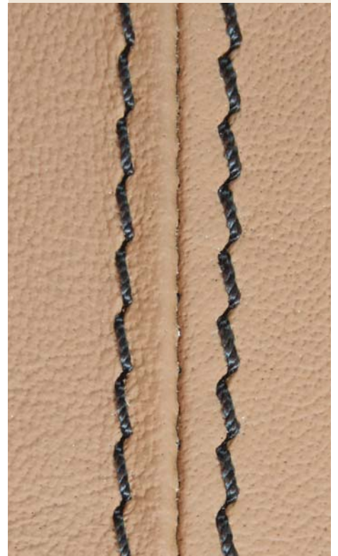
UNEVEN SEAMS PRODUCED BY THE LEFT AND RIGHT-HAND NEEDLE
